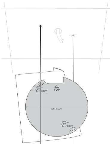
2. Use an appropriate size drill to mark the holes using the mounting template.
